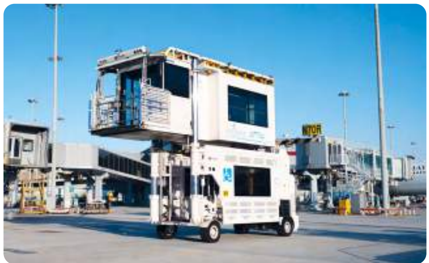
A new ambulift adds convenience for passengers with limited mobility by helping them board or disembark from aircraft.
