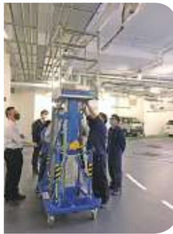
◀ Mobile elevated working platform for work at height use 用於高空作業的流動式升降工作平台
