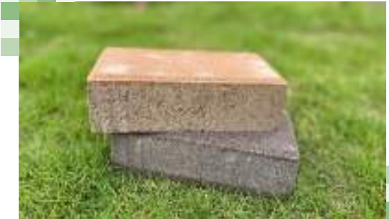
Trial on making eco-paver by upcycling spoil ballast generated from East Rail Line ballast replacement project.
