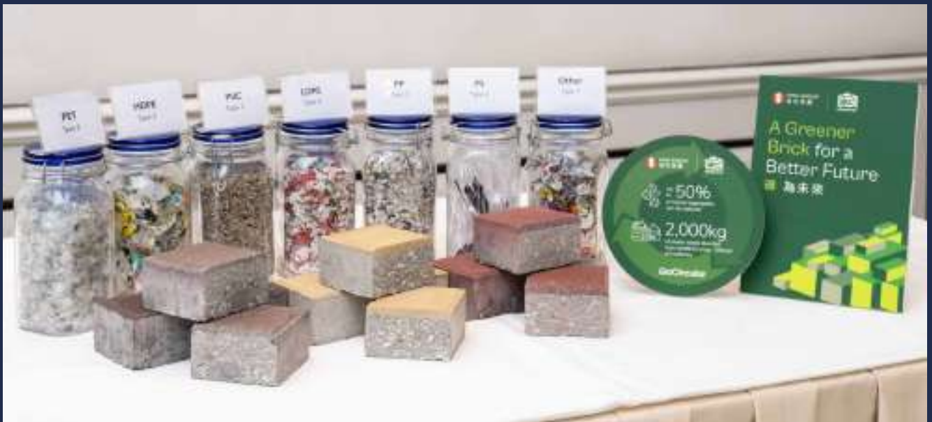
The solution upcycles all seven types of plastic waste, including mixed and composite plastic that are currently impossible to recycle, into sustainable construction materials.
