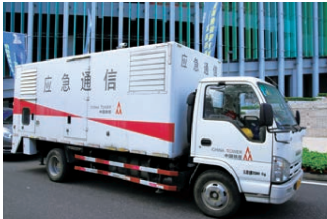
▲ Emergency support power supply vehicles
