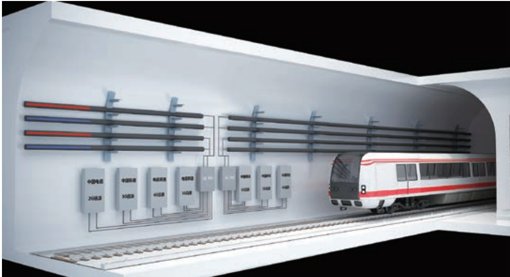
Leaky Cable Cross-Polarization 4T4R Solution Improves 5G Performance of Subway Tunnels
