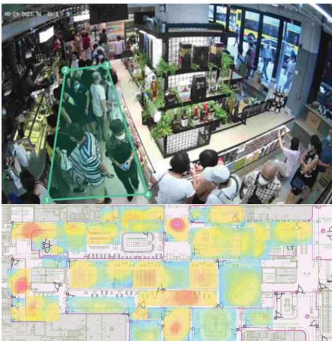
Adopting the BIM-Facility Management system, Central Market can now monitor the visitors traffic and analyse their engagement data for effective crowd management and better customer experience.
